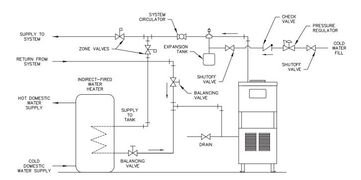
Figure 3.7: Typical Piping with Indirect-Fired Water Heater
